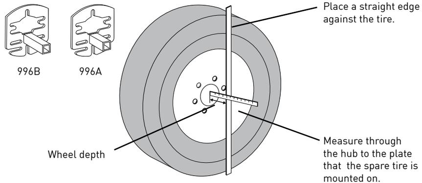
If the wheel depth (distance from spare tire mounting plate to outside of tire) is between 5" and 7-3/4" you must use Base Plate 996B. If the wheel depth is between 2-1/2" and 5-1/4", use Base Plate 996A. Measure through the hub to the plate that the spare tire is mounted on.
